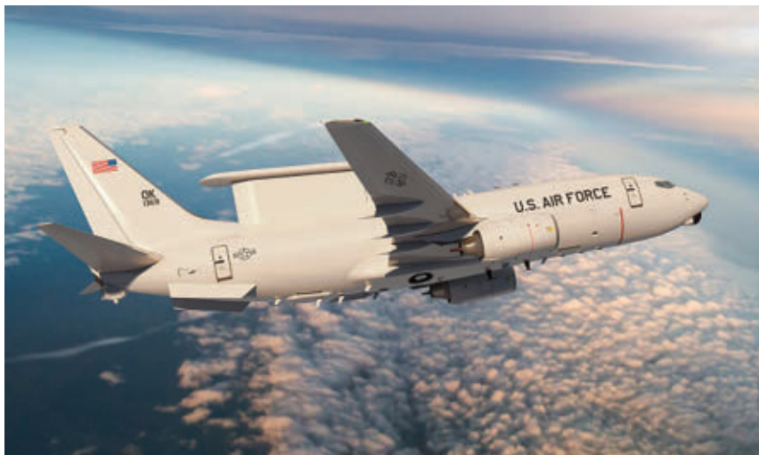
The E-7A is based on the Boeing 737-700ER long-range single-aisle passenger jetliner, and will be for simultaneous air and sea search, as well as combat air traffic control.
