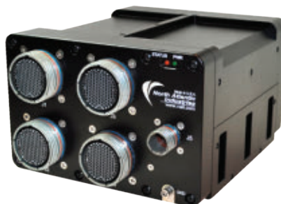
▲ The North Atlantic SIU35 3U CompactPCI sensor interface unit is being integrated into the Raytheon for the Raytheon Lower Tier Air and Missile Defense Sensor (LTAMDS).
